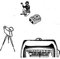
Incident Light Measurement: Move the converter slide (10) so that the spherical diffuser is centered over the round window. The Luna-PRO is ready when the converter slide has clicked into position. Point the Luna-PRO from the subject towards the camera, as indicated by the arrow in the illustration.
